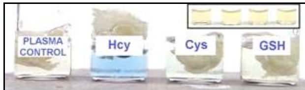
Figure 4.3. Selective detection of Hcy in human plasma without prior deproteinization. (added thiol left to right: none, Hcy, Cys, GSH. Inset: samples before heating.)
