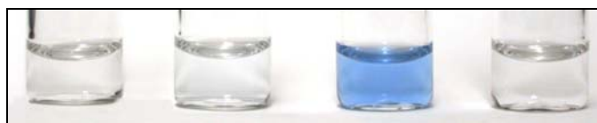
Figure 4.1. Selective color change in response to Hcy in solutions of MV^{2+} . (Left to right: no added analyte, Cys, Hcy, GSH)
